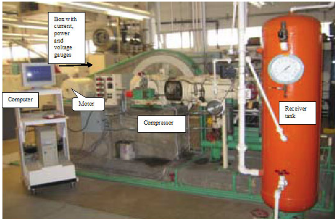
Figure #2 Reciprocating Air Compressor Test System
